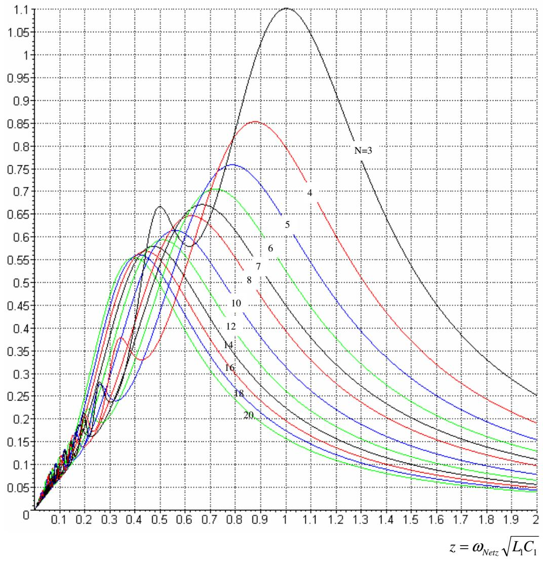
$$\frac{i_{L1}^{eff}}{u_0^{eff} \omega_{Netz} C_1} = \frac{i_{trafo}^{eff}}{u_0^{eff} \omega_{Netz} C_1} \quad \text{ohne Blindstromkompensation}$$
